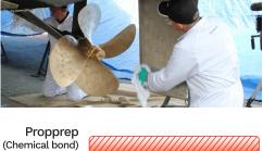
Wipe down the surfaces with **Propprep** wipes, immediately wiping with a clean, dry rag. Repeat until there is no residue left on the cloth. Propprep contains no corrosion inhibitors, so proceed with Step 3 as soon as possible, but definitely within 4 hours.
