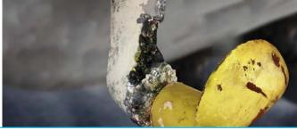
AC stray current causing colour change and paint deflection to metallic surfaces. Can be seen by premature Propspeed failure, high levels of growth and/ or unusual anode wear.
